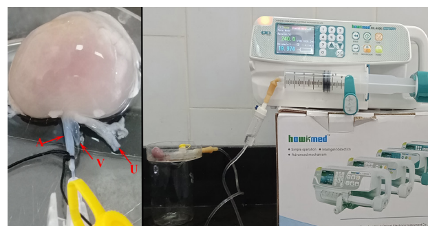
Fig. 1: A photograph showing the decellularization device assembled by connecting the cannulated left rabbit kidney to hawkmed® HK-400II syringe pump (Shenzhen Hawk Optical Electronic Instrument CO., LTD) which infuse fluids at certain given rates. On the left, a closer view showing the IV cannula inserted in the renal artery (A) while the renal vein (V) and ureter (U) are free.
